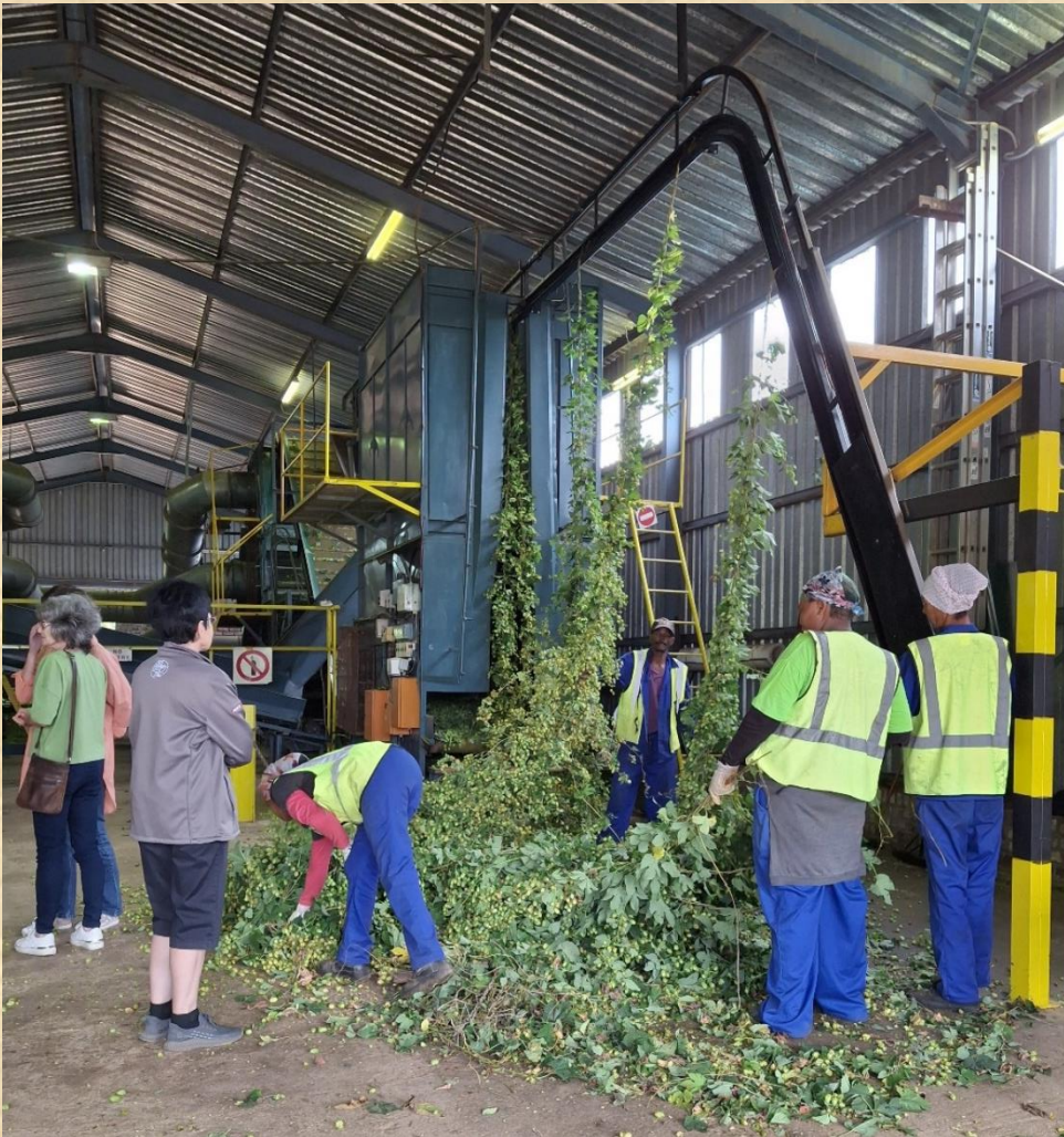
Above: The hops processing plant where the cones are separated from the rest of the plant material.
