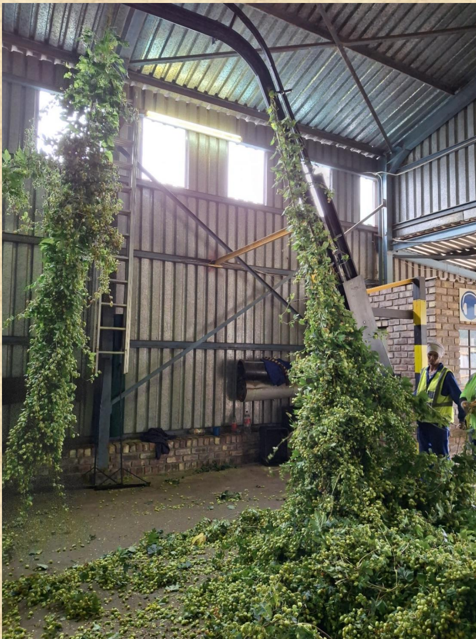
Above: The hops is fed into the machines by hand to remove the cones.
