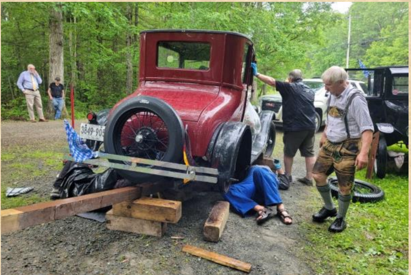
Above and below: Rear axle removal and repair.
