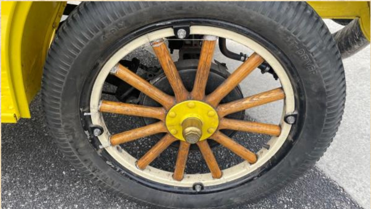
Above: The temporary fix to try to tighten the loose spokes.
