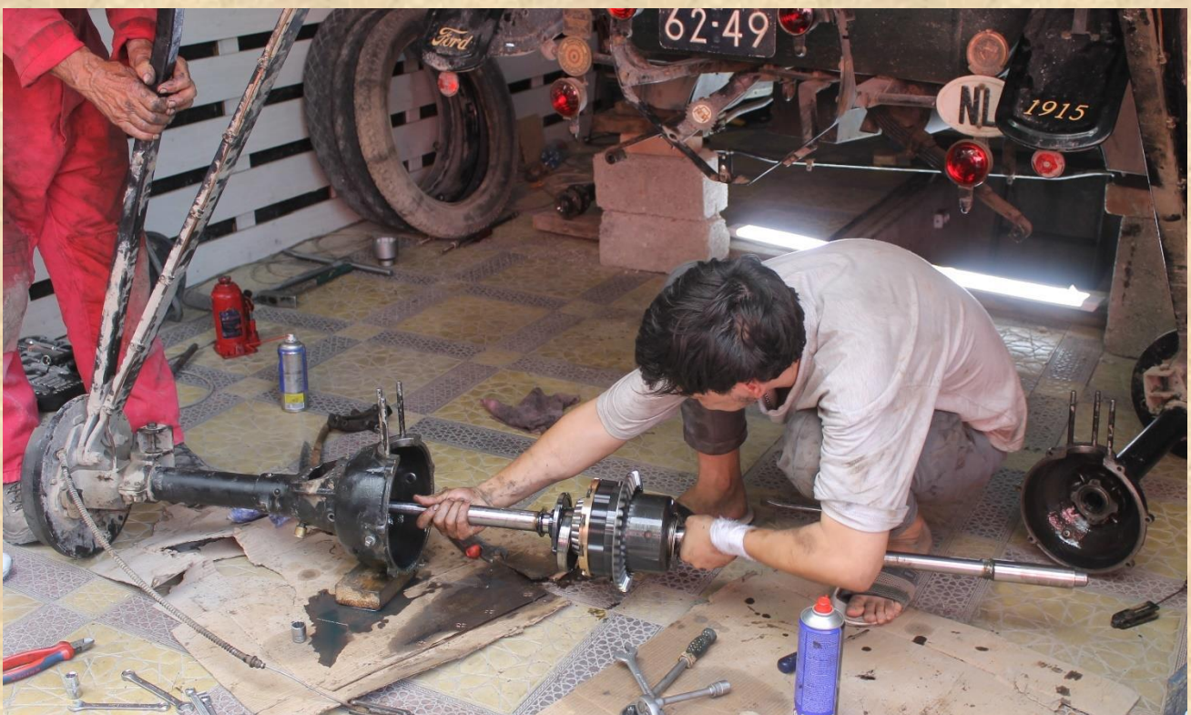
Above: Repairs to the rear axle of the Model T Before leaving Dushanbe.
