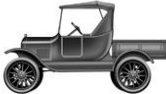
Roadster Pickup - Open Car - no side windows, front seat only, rear bed for cargo.
