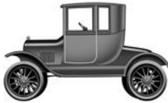
Coupe - Closed Car - two doors, enclosed interior with front seats only, side glass windows.
