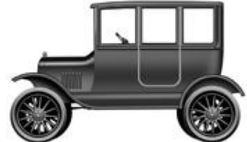
Centerdoor Sedan - Closed Car - enclosed interior with front and rear seats, side glass windows, door positioned in the center of the body.
