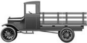
TT Truck - enclosed interior, adaptable chassis/rear cargo area, worm drive rear axle )
