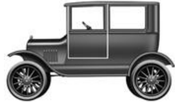
Tudor Sedan - Closed Car - two doors, enclosed interior with front and rear seats, side glass windows.
